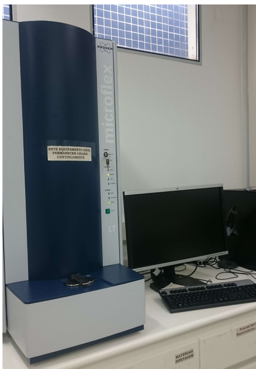
Figura 3. Espectrômetro de Massas do Tipo MALDI-TOF ( Matrix-Assisted Laser Desorption/Ionization Time-of-Flight Mass Spectrometry ), Modelo Microflex, Marca Bruker-Daltonics®
