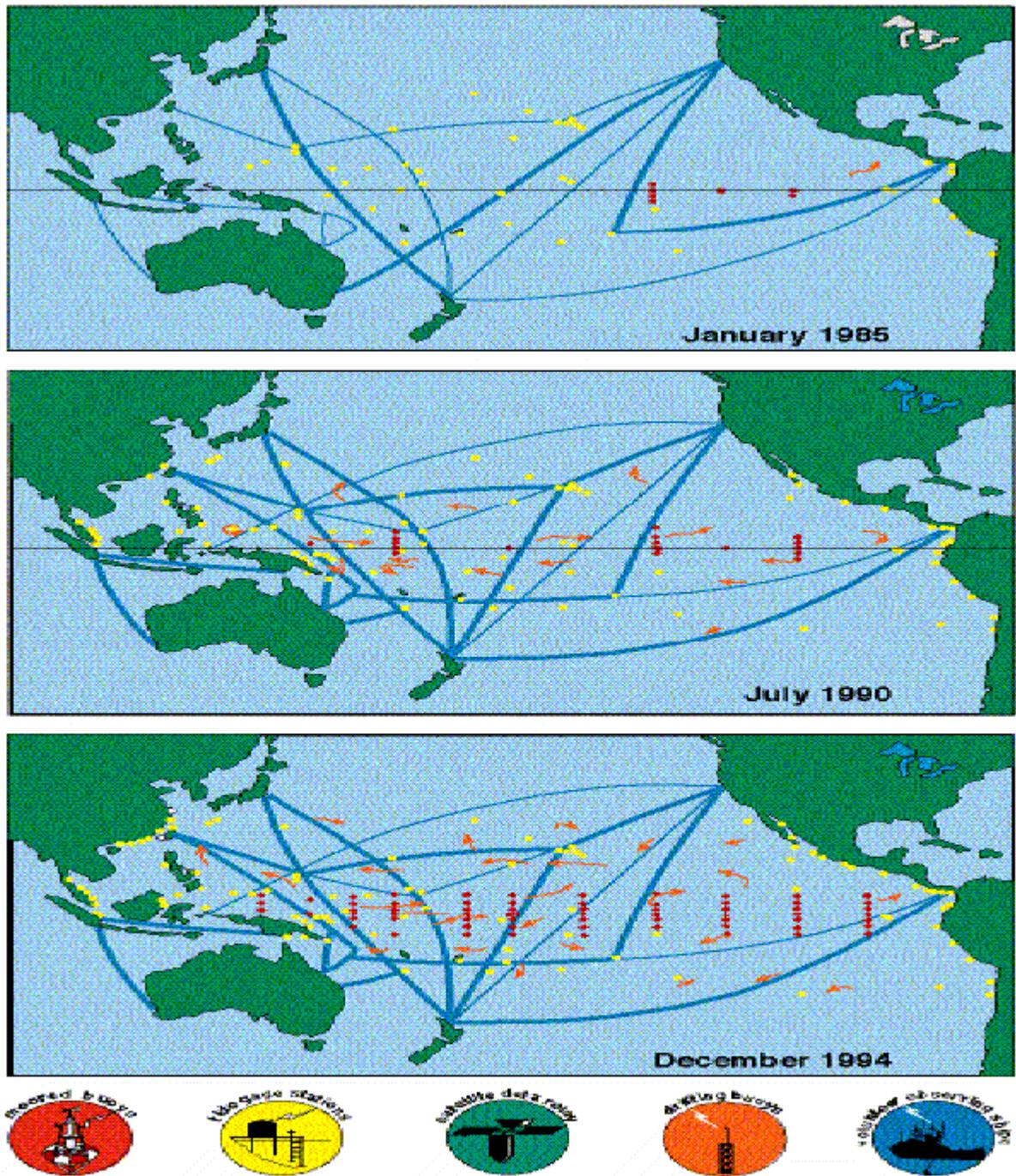
**Figure 5.** The improvement in the in situ observing system in the Pacific from 1985-1994: January 1985 (top), July 1990 (middle), December 1994 (bottom). The “pluses” show moored buoys, the “arrows” drifting buoys, the “lines” ships, and the “dots” tide stations.
