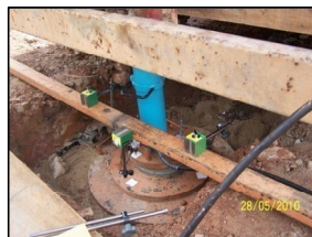
Step 5: Gauges placement
