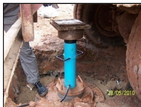
Step 4: Hydraulic jack placement
