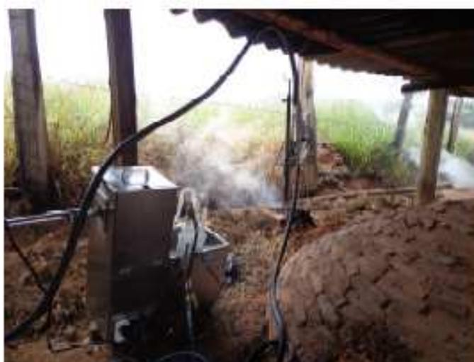
Figure 1 – Sampling system for PCDD/Fs
